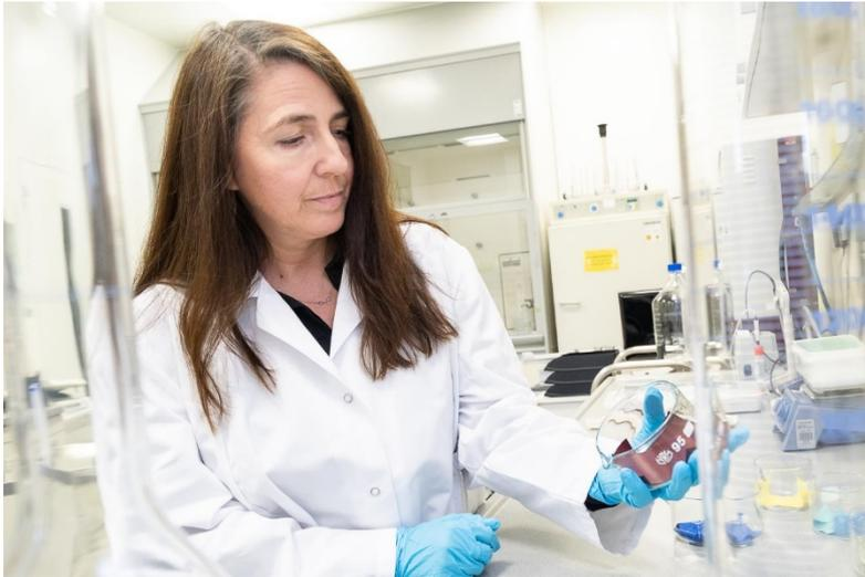
BU: Preparation of textile samples with skin simulating gel (Photo FKTe.V.)
